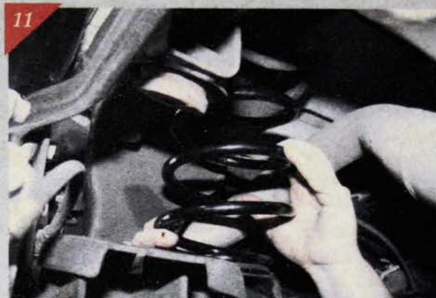
Replacing the coils is as simple as pulling the factory coils out of their perches and dropping the McGaughy's drop springs into place. The shocks will hold the shorter springs in place.
