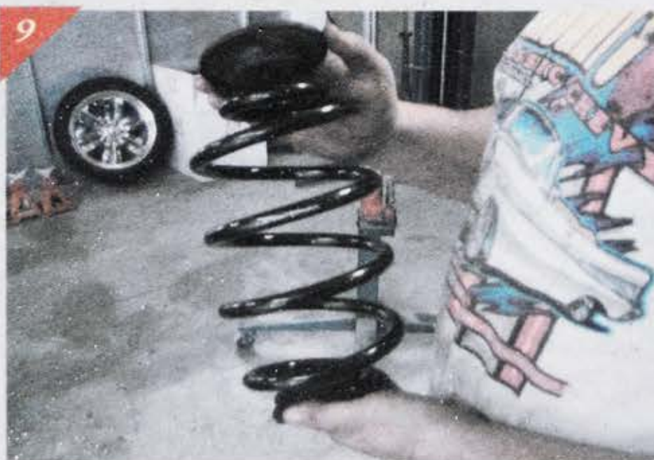
McGaughy's rear drop kit is also an easy install. The original coil springs can be replaced with these McGaughy's springs, and the shocks are replaced with McGaughy's performance shocks, which help maintain a good ride.
