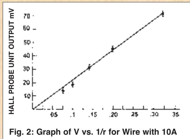
Fig. 2: Graph of V vs.  $1/r$  for Wire with 10A
