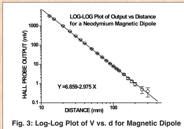
Fig. 3: Log-Log Plot of V vs.  $d$  for Magnetic Dipole
