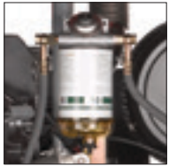
High-efficiency multi-step fuel filtration with water separator
