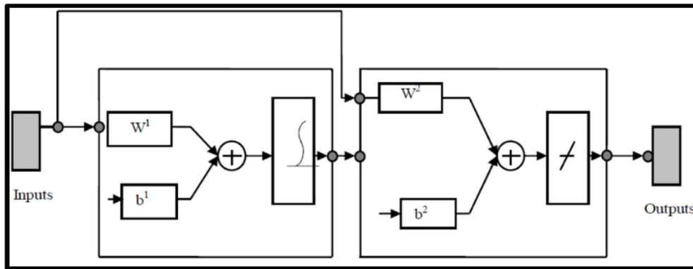
Fig.4: Cascade feed-forward neural network
