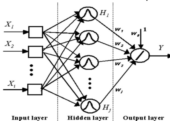
Fig.3: Radial basis function neural network
