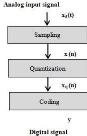
Fig.2: Applying digital signal processing operations on an analog signal
