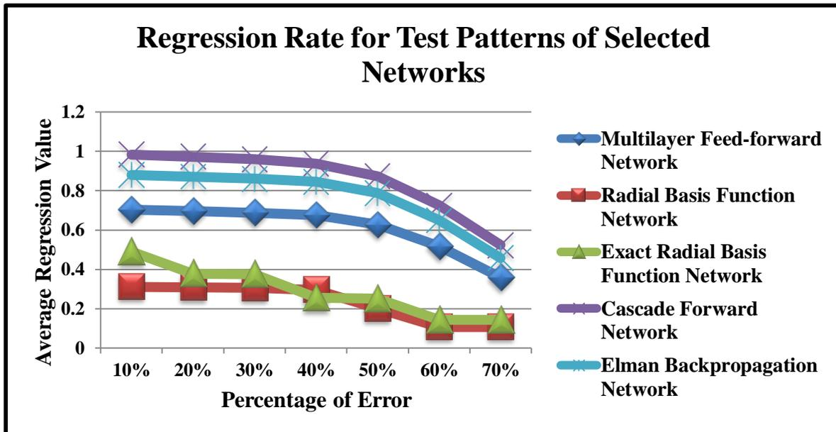
Fig.7: Comparison of regression values of testing patterns for all selected neural network models
