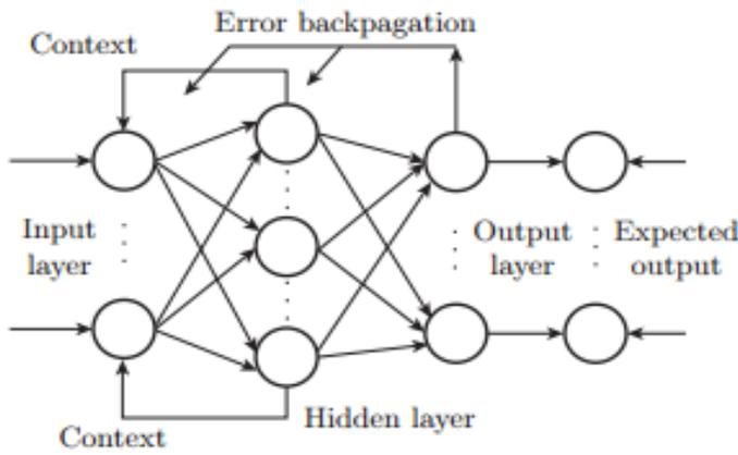
Fig.5: Elman back propagation neural network
