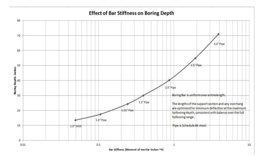
The big problem with hollowing/boring, is the length of the boring bar "hanging" over the tool rest. The more overhang, the more leverage that the handle has to overcome and the more the bar will flex.
