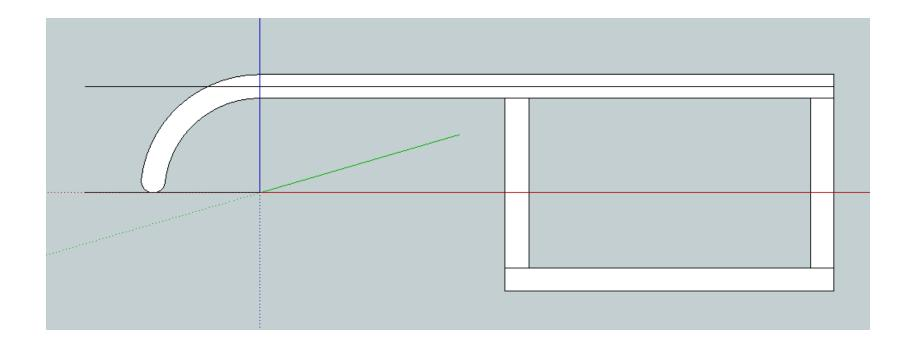
The width of the "outrigger" and "trap" will limit the horizontal motion of the boring bar. An articulated boring bar may have more movement, but the standard trap can be remounted in different locations for the desired movement.
