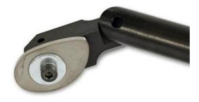
The cutter is mounted at a 45 degree angle and since it is high speed steel, it requires more frequent sharpening, but since it is used just for the finish cut, that is not a problem.
