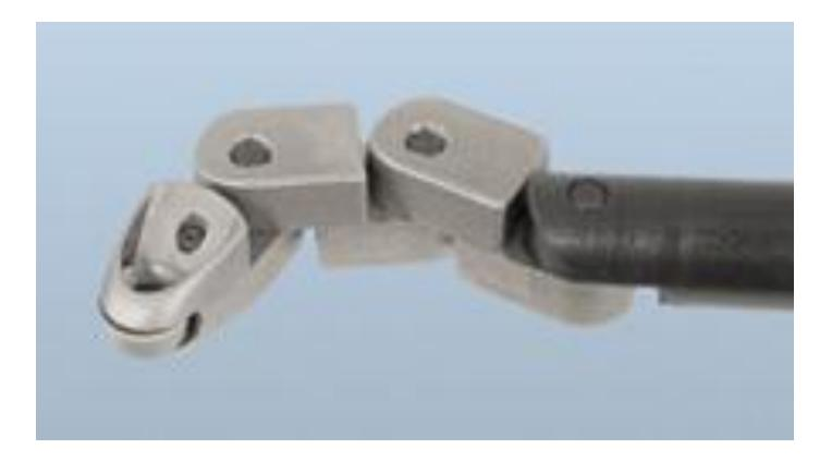
First, it has a carbide cutter which is supplied by Mike Hunter. Carbide lasts far longer than high speed steel, which is vital when it takes several hours to hollow a large vase.
