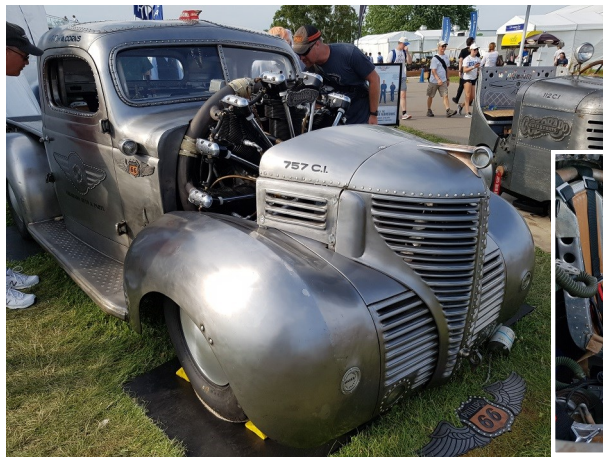
1939 Plymouth truck, complete with Jacobs radial aero engine & rear booster rocket
