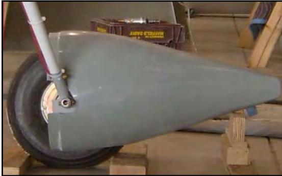
**Note:** A variety of different wood pieces are very helpful when fitting the wheel pants as the help to position the correctly while fitting.
