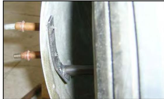
14. Transfer the out line of the bracket to the outside of the pant.
