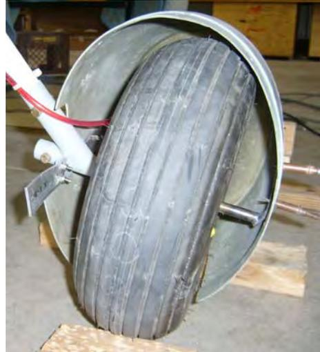
25. Now that the wheel pants are fitted to the mounts carefully mark where they must be trimmed to add clearance for operation.
