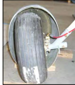
8. Slide the out board wheel pant bracket in place in the axle.
