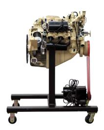
H-HMMWV-6.2-CA Humvee Engine Cutaway on Mobile Stand
