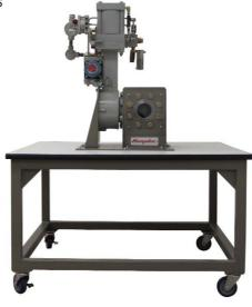
H-MVOT-X Motorized Valve Operator Trainer Cutaway
