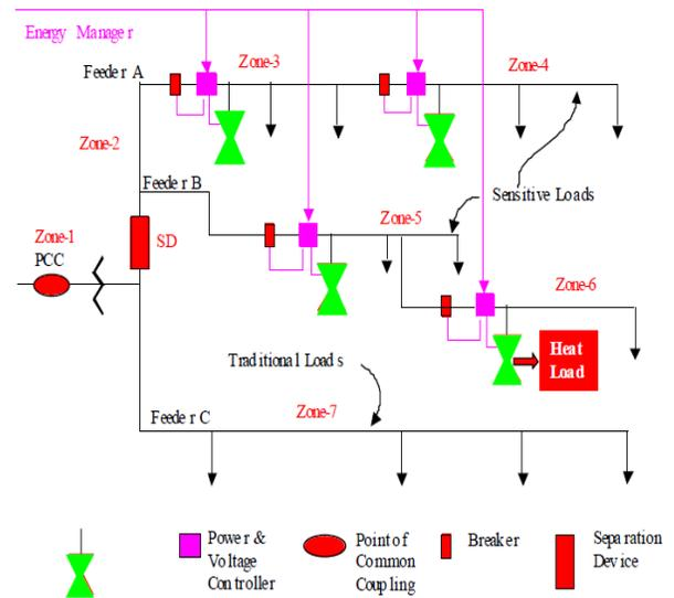
Fig.2 Microgrid Architecture
