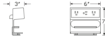
3 simplex receptacles (E)
