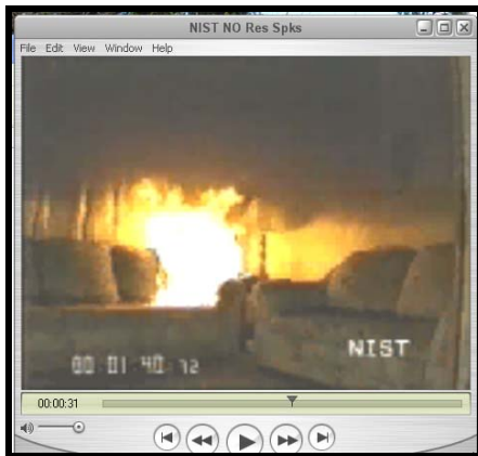
1 minute 40 seconds Smoke hot layer clearly visible
