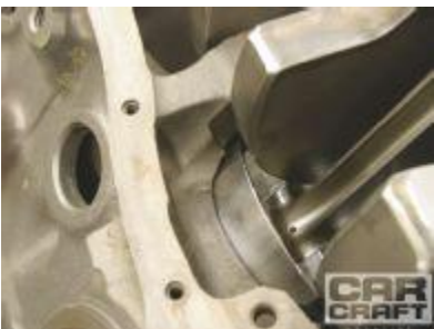
Look closely and you'll notice that our first-choice 4.500-stroke Scat crank pulled virtua
