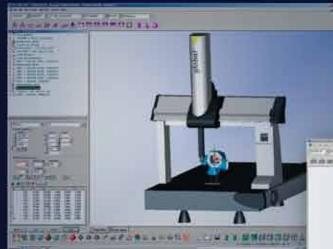
PC-DMIS software takes full advantage of Global scanning capability. In the example shown, the machined flange surface is being scanned for flatness; PC-DMIS allows for the specification of scan paths, shown as the yellow curvilinear line below.
