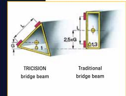
Global's TRICISION extruded triangular cross section bridge beam enhances dimensional stability for superior metrology performance.
