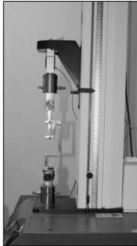
Figure (5): Instron universal testing machine with metallic assembly attached.
