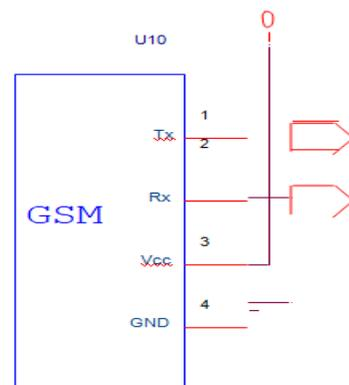
SIM900 is a Tri-band GSM/GPRS engine that works on frequencies EGSM 900 MHz, DCS 1800 MHz and PCS 1900
