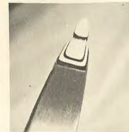
Groves' typical narrow tip has been reinforced with fiberglass overlays.
