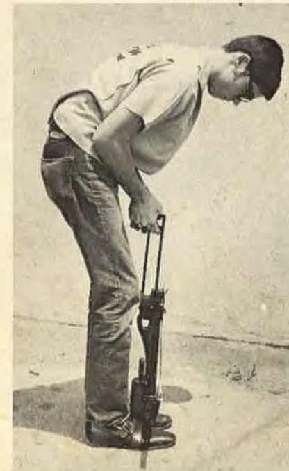
Sliding stock pulled all the way to the rear, the bow is cocked and now is ready for the bolt to be nocked.
