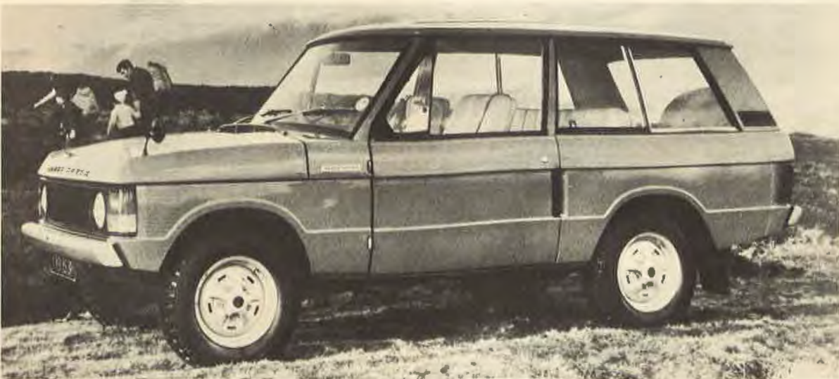
Range Rover is deluxe version of familiar Land Rover, goes 90 mph on highways, slow but sure elsewhere with 4-wheel drive; seats five.
