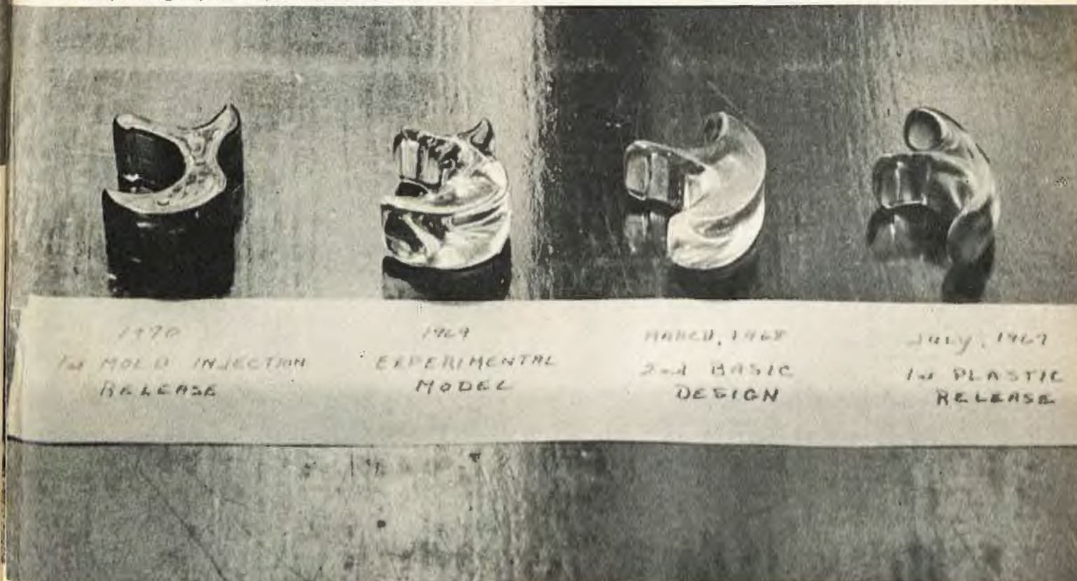
From right: the development of the plastic release is shown, coming to final conformation for production type.
