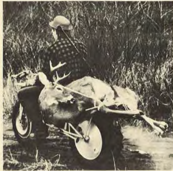
Trail-Breaker features 2-wheel drive, water-tight engine, gas/water storage in wheels — phenomenal capability.
