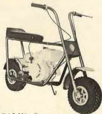
The "Flea," by K&P Mfg. Co., goes up to 30 mph with 4-stroke, 3.5-hp Tecumseh engine, has automatic centrifugal clutch.
