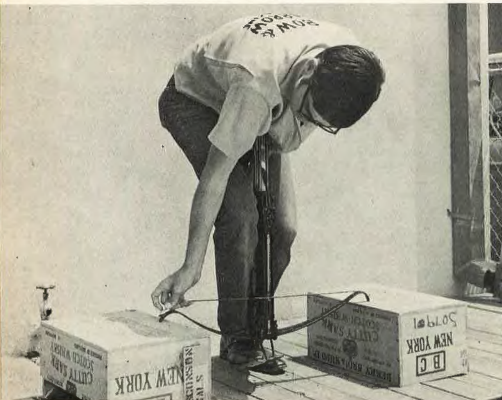
Stringing the bow is accomplished with two boxes of equal height, bending limbs until bowstring reaches the nocks. Steve Bennett illustrates how it is done.
