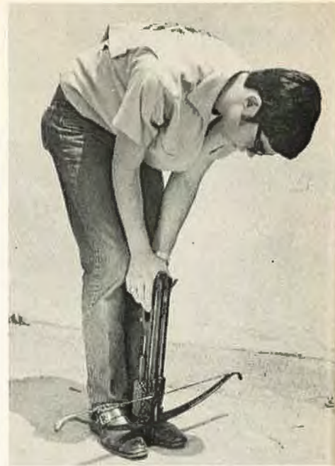
Sliding stock picks up the bowstring, when pushed to the forward position. It cocks automatically by pulling stock to rear of the 140-pound bow.
