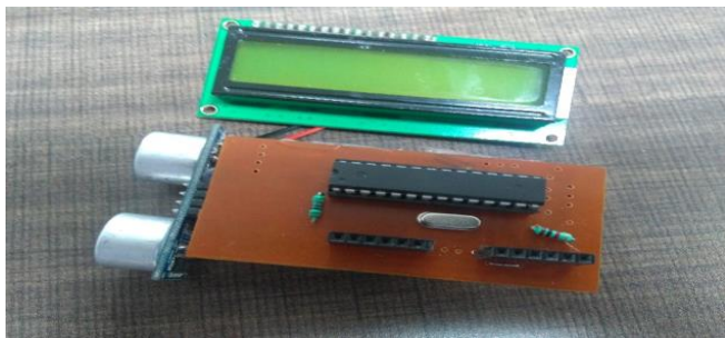
Figure 11. Measurement using AVR Controller
