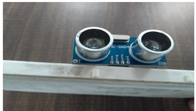
Figure 1. Ultra-Sonic Sensor HC-SR 04.
