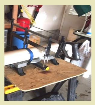
Secure the tube to the miter saw assembly with a cam strap; it snugs the cylinder down even better than a vice.
