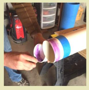
Paint on the primer and then the second part of the 2-part contact glue as the product directs. Put the cap in place; the bond will harden almost instantly. П
