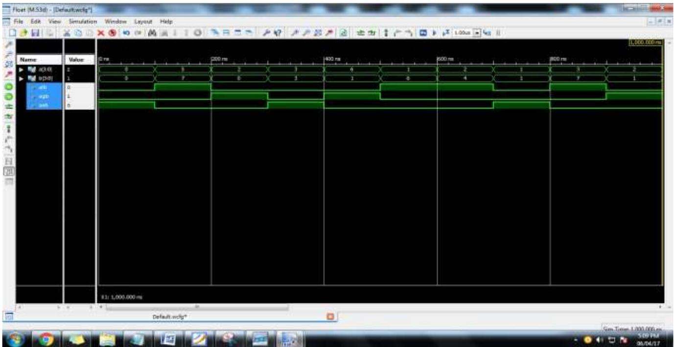
Fig. 2. Output waveform of 4 bit reversible comparator
