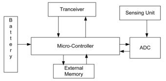
Fig.1: Components of a wireless sensor node
