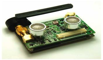
Fig.2: Wireless sensor node
