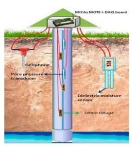
Fig.7: Landslide Detection
