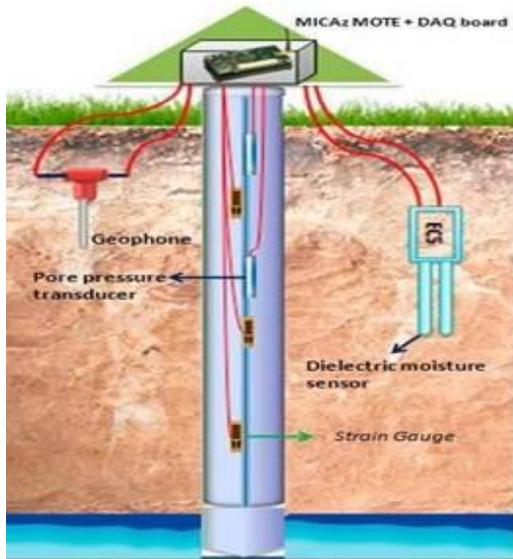
Fig.7: Landslide Detection
