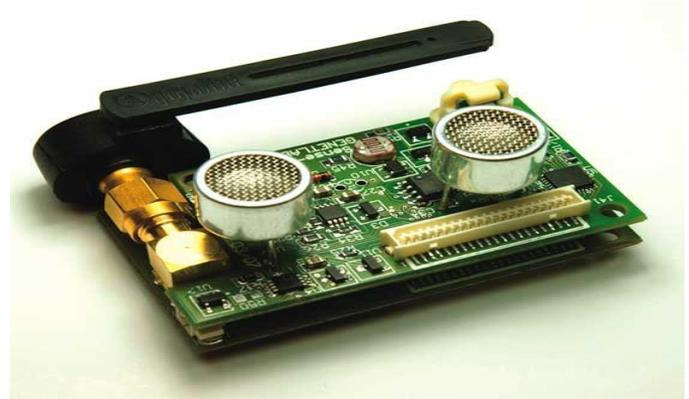
Fig.2: Wireless sensor node
