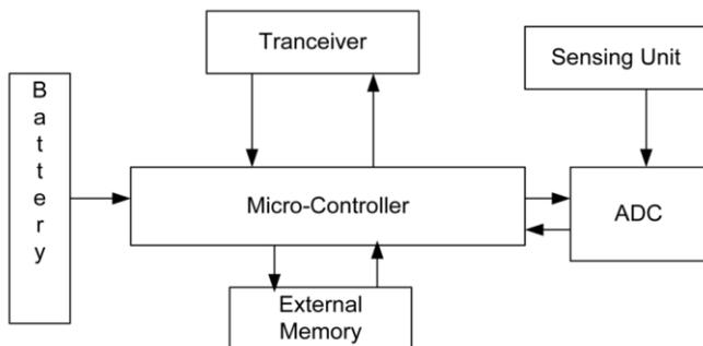
Fig.1: Components of a wireless sensor node
