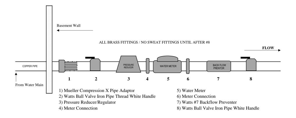
Please follow the diagram above and make sure to have all the necessary fittings and connections. Once the set up is complete, you can call the Village Clerk's Office at 845-292-2250 to request an appointment to have the set up inspected by Water District personnel. If the requirements are met, the water meter will be installed. Thank you!
