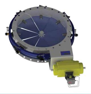
Predominantly used on fan inlet applications, offering an enhanced level of flow and pressure control, with multiple blades arranged around a central hub. This enhances the performance of the fan by introducing swirl into the fan inlet providing an efficient method of control.
