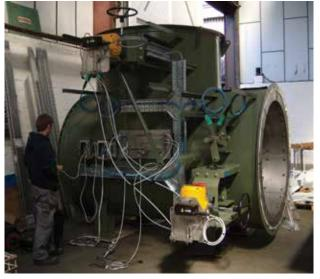
As an alternative to a flap diverter, multilouvre dampers can be built into a T-Duct section and linked to provide an effective inlet / bypass solution. These can be incorporated with a guillotine to provide a fully integrated inlet/bypass/isolation solution. Seal air systems can be added to any of our diverters to provide 100% sealing efficiency.
