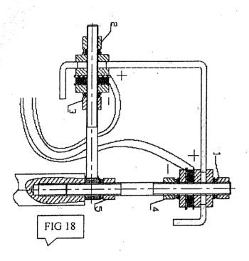
pre-pressure of the press sensor (use torque wrench to lock and the torque is 40NM) There are glass glue coat on the surface of the press sensor and the normal installation result of the piezoelectric ceramics disk of the sensor is the IR should be larger than  $50M\Omega$ .
