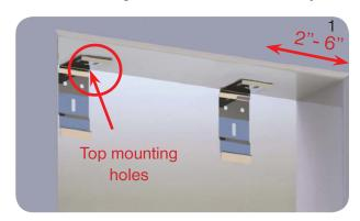
**Be Advised:** For Cassette systems greater than 4 ft, you will be supplied with additional mounting brackets. Evenly space these brackets dividing the total width of window opening by the number of brackets supplied.
