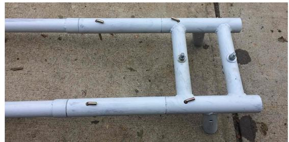
Complete the top section assembly of the GoHoist unit by joining the 48" crossbeam sections together and then placing the other shoulder section on the crossbeam assembly and securing with locking pins.
