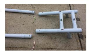
Step 3. Insert the two (2) ends of the crossbeam segments into the open end of the two (2) extension segments, lining up the holes and inserting locking pins as shown to the right.
