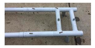
Complete the top section assembly of the GoHoist unit by joining the 48" crossbeam sections together and then placing the other shoulder section on the crossbeam assembly and securing with locking pins.
