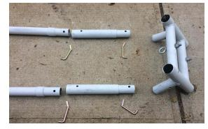
Step 2. Insert the two (2) extension segments into the shoulder section as shown to the right. Place two (2) locking pins securing the shoulders to the extension segments.
