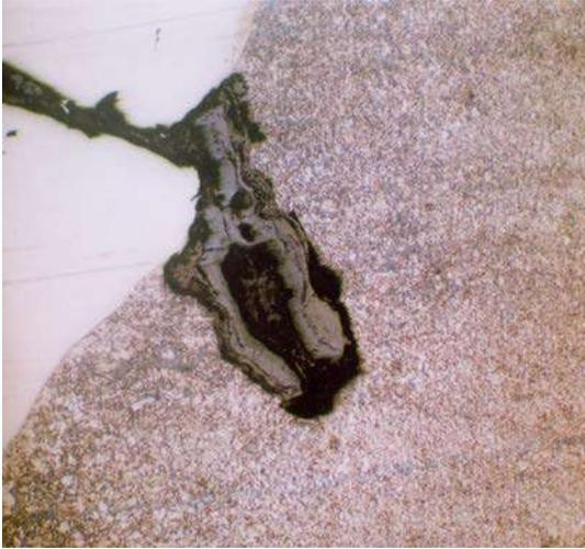
The crack has initiated at the HAZ of the carbon steel pipe and has propagated into weld metal
