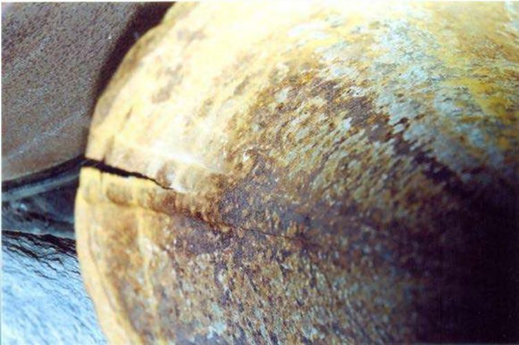
In the internal surface there was localized corrosion in the form of a canal throughout the length of the pipelines. There is heavy metal loss in the canal resulting in the formation of slits and holes.
