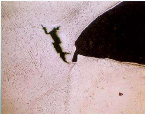
Near the tip of the main crack another microcrack was also seen at the weld metal This crack lies on hard zone typically found in dissimilar metal welds
