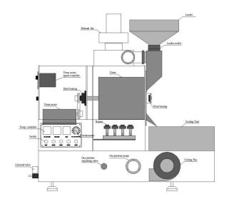
THE BC-3 MD IS A HEAVY DUTY ROASTER BUILT WITH A CARBON STEEL BODY WITH APPROVED POWDER COAT HIGH TEMPERATURE BODY IN BLACK. THE HOUSINGS COME IN A CHOICE OF 4 COLORS (Gold, Rose Gold, Black Titanium & Stainless) In two type finishes (MIRROR or MATTE) TWO EXHAUST PIPES COMES OFF THE BC-3 AT 3" AS SHOWN BELOW AND CAN BE EXHAUSTED OUT OF BUILDING SEPARATELY OR CONNECTED WITH A BLAST OR BACKDRAFT DAMPER
