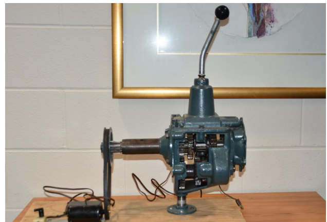
Bob Butek made this working cut away transmission
