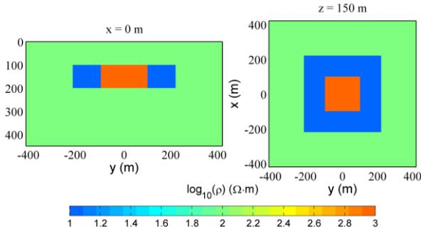
**Figure 3.** A simple 3D model. The low and high resistivity body is 10 Ω·m and 1000 Ω·m, respectively. The background resistivity is 100 Ω·m.
