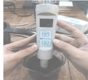
Figure 6: Set-up measuring the pH nanofluid
