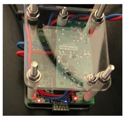
If no lights come on check wire connections. If all are properly connected then data logger could be damaged or defective.
