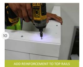
Fasten CORNER BRACKETS (true yellow label) to the TOP CORNER RAILS for added reinforcement.
