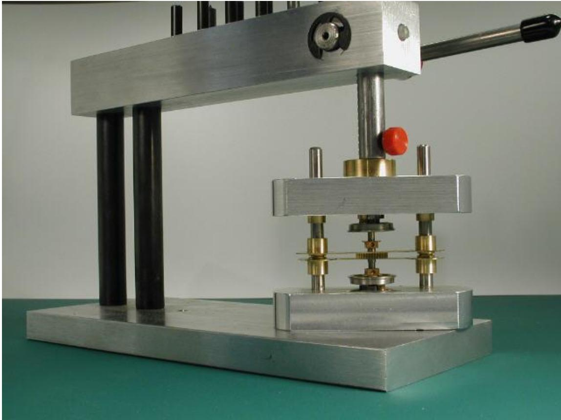
Photo 9. The driver assembly and jig is now placed in the NWSL Sensipress, and the assembly is pressed home. Is this cool or what ?!!
