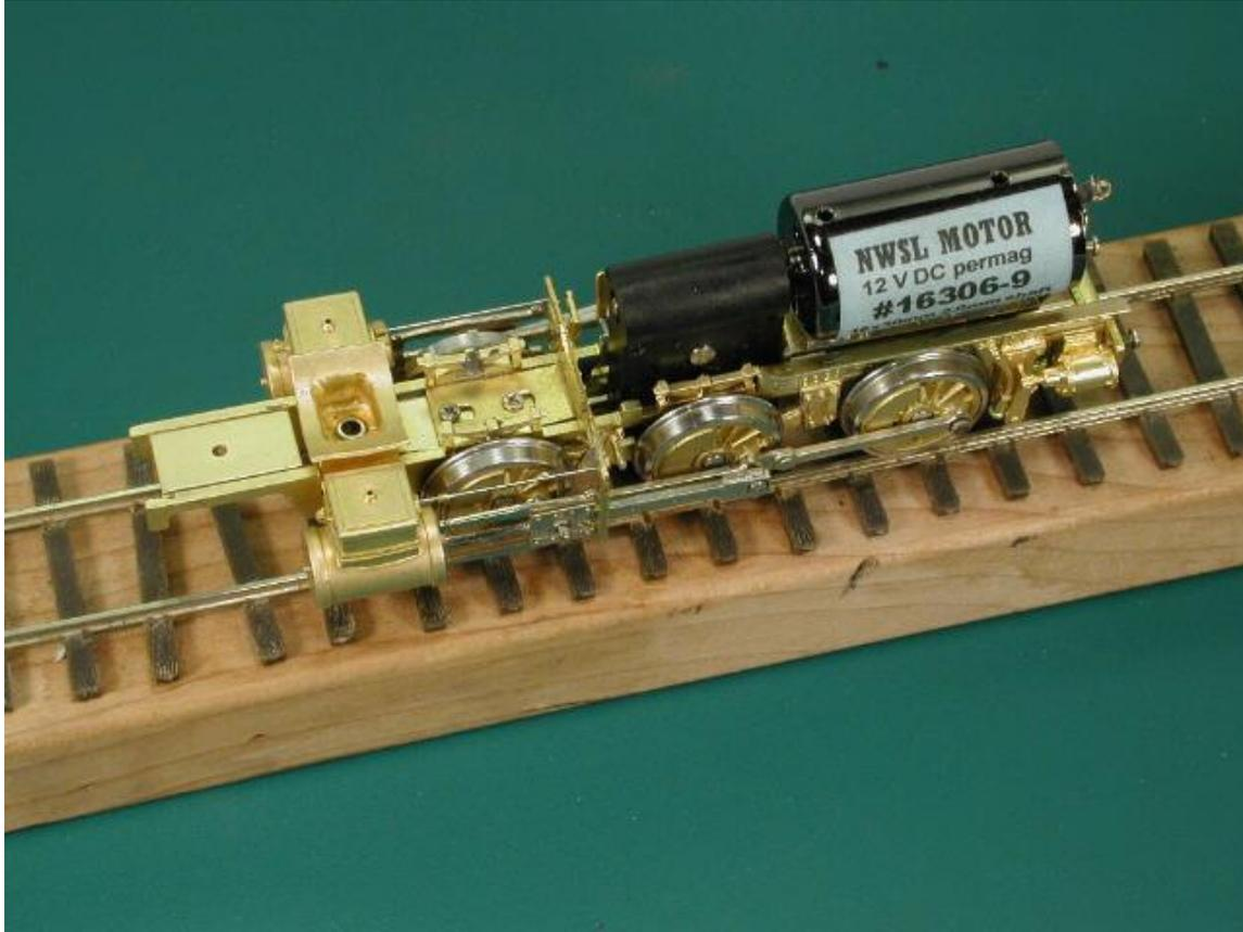
Photo 14. Before attaching the gearbox to the mechanism, a small amount of silicone grease was applied to the gears. After attaching the gearbox and torque bar to the mechanism, a small amount of oil will be placed on all bearing surfaces: crosshead guides, side rod screws, etc.. Next we will prop up the mechanism on a couple of pieces of wood to clear the drivers, apply a few volts of DC, and run the locomotive in for about 15 minutes in each direction. Perfection !!!
