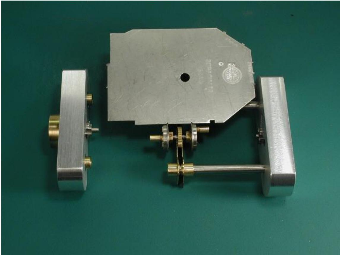
Photo 10. The Quarterer has been opened up and the gauge of the wheels is checked. It may be necessary to “tweak” the drivers slightly, by using either the NWSL Puller and/or the NWSL Sensipress to ensure perfect gauge. Just remember to work carefully, so as to keep the fit tight.
