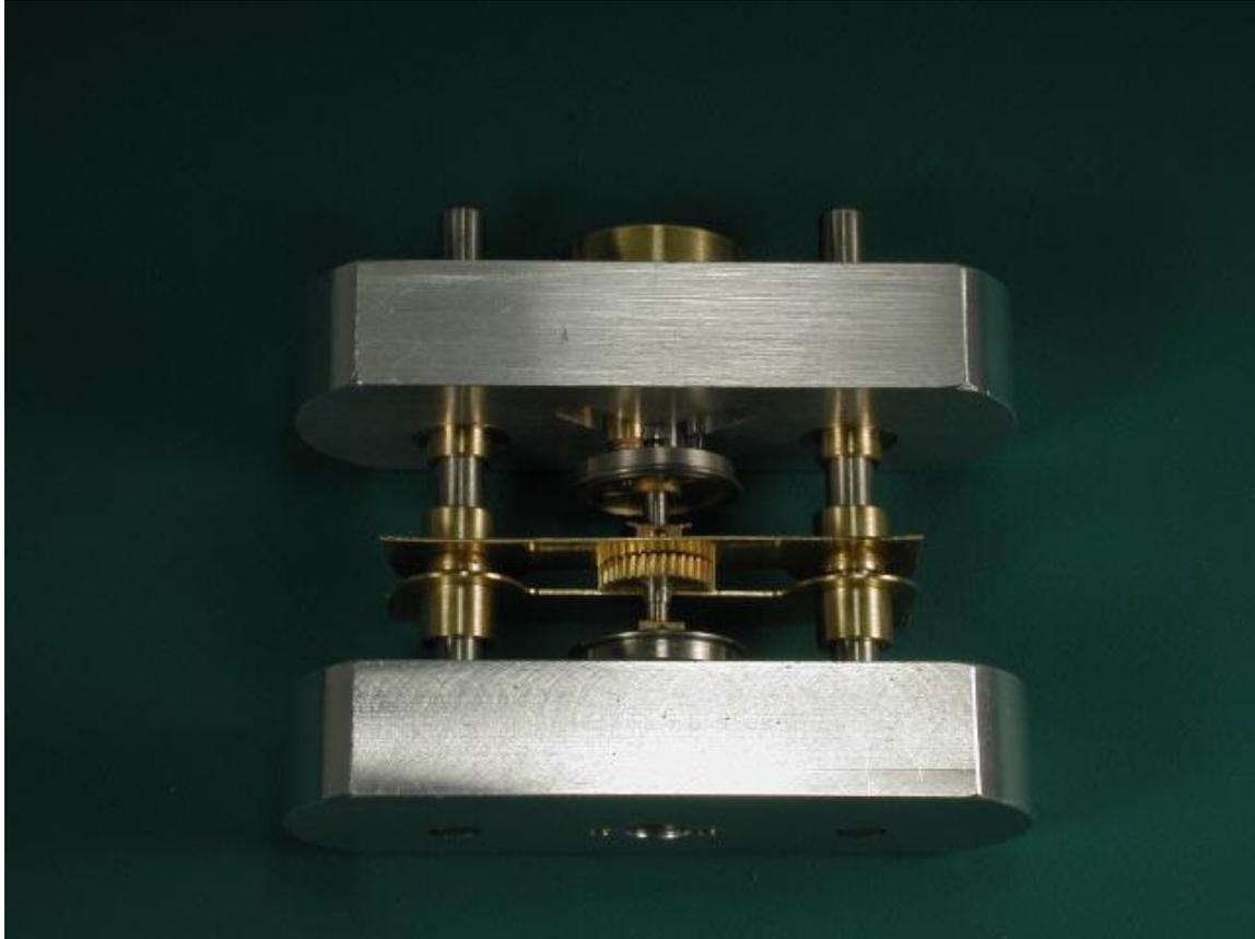
Photo 8. Another view of the drivers and geared axle aligned in the jig. Careful examination of the photograph reveals the insulated driver on the bottom, collets forward (right), bearing, 3.0mm alignment plate with notch up, gear, 3.0mm alignment plate with notch down, bearing and uninsulated driver on top with collets back (left).
