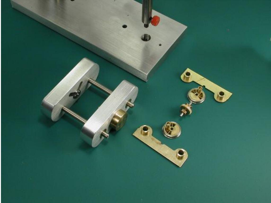
Photo 6. The bearings – flanged side out – have been placed on the axle, and the drivers and the geared axle are now ready to be mounted in the Quarterer. Two sets of brass alignment plates are required for this project – 3.0mm for the second axle, and 2.5mm for the first and third axles. This is necessary because of the differing axle diameters...remember?
