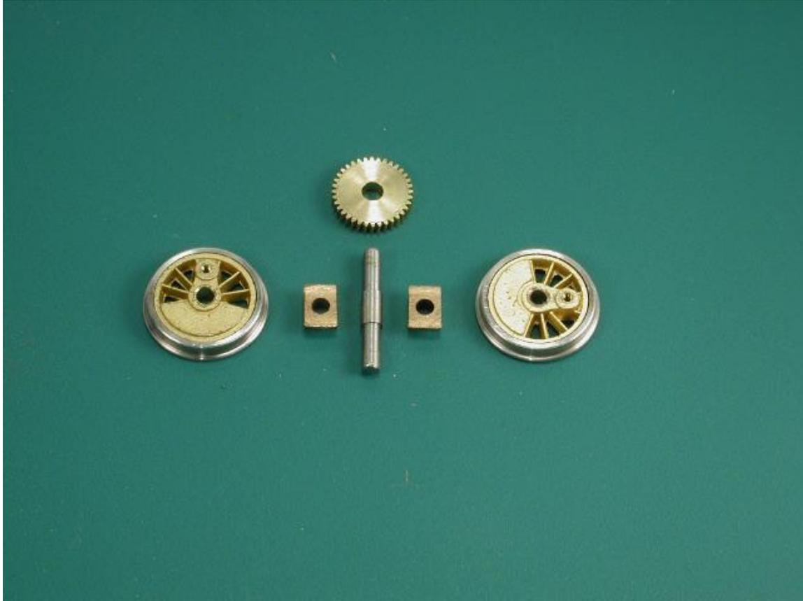
Photo 4. Using the NWSL Puller, both wheels and both bearings have been removed from the original geared axle. The new axle and gear are pictured, along with the drivers and bearings.
