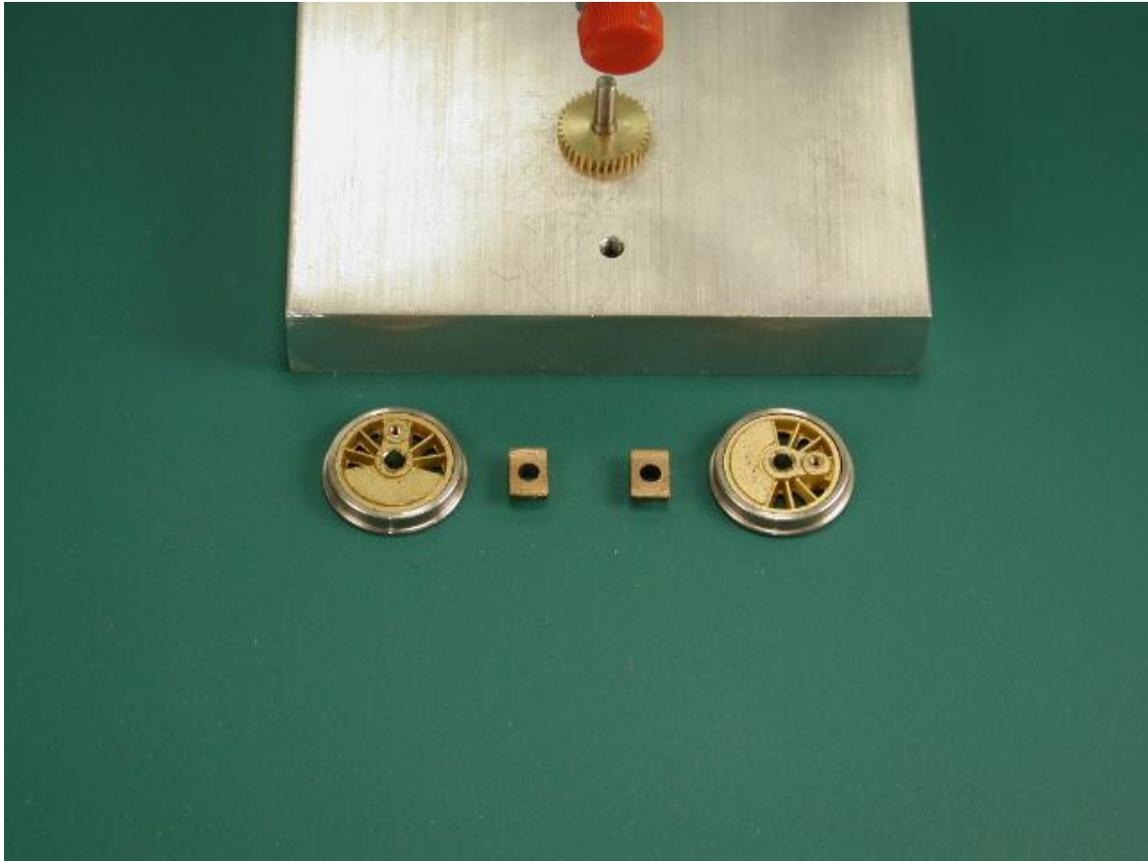
Photo 5. Using the NWSL Sensipress, the new gear is pressed to the exact center of the new axle, true and square.
