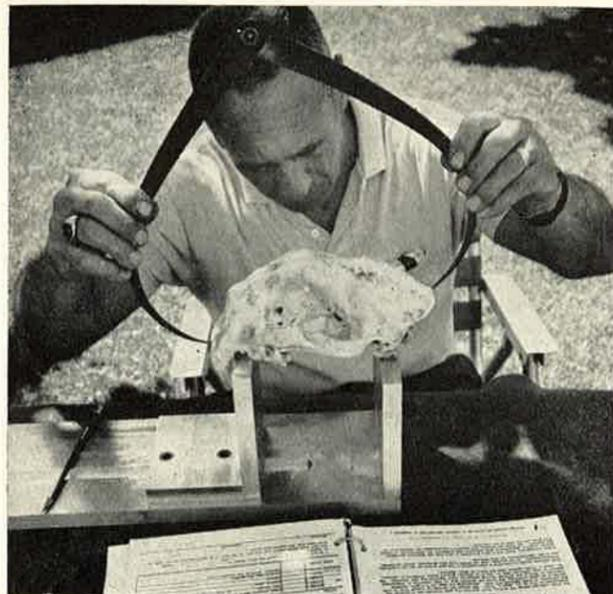
**ACCURATE BUT TRICKY**—A good grade of outside callipers with inward sweep ends that come to a needle point will measure skull lengths and widths accurately if held in proper alignment
