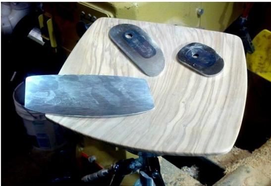
The large curved scraper is the one I usually use on the top. This will take out ripples in the dish and leave the surface very smooth. Always scrape downhill.
