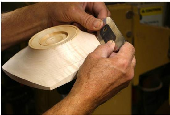
The smaller scrapers are excellent for the bottoms of these little platters. A flat or gently curved edge can be used on the curves of the bottom and to remove all tool marks from the wings.
