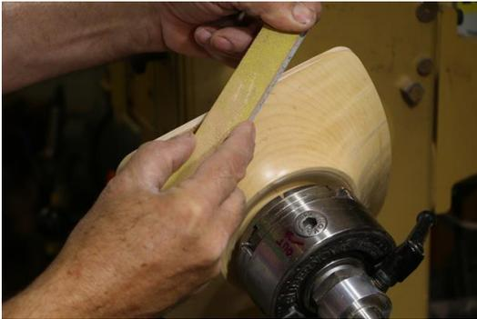
Shape by hand with files, sand paper, or sanding sticks. Minor chips on the edges can be removed. The rim might be rounded, angled, or thinned. This is also the best time to round the corners slightly if desired.
