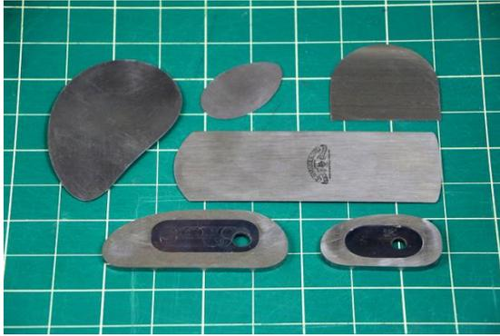
I use handheld scrapers with the lathe off to remove any tool marks in the center of the recess and on the large curve on the bottom, all the way to the corners of the wings. This requires much less sanding, usually starting with 220 or 320 grit or finer.
