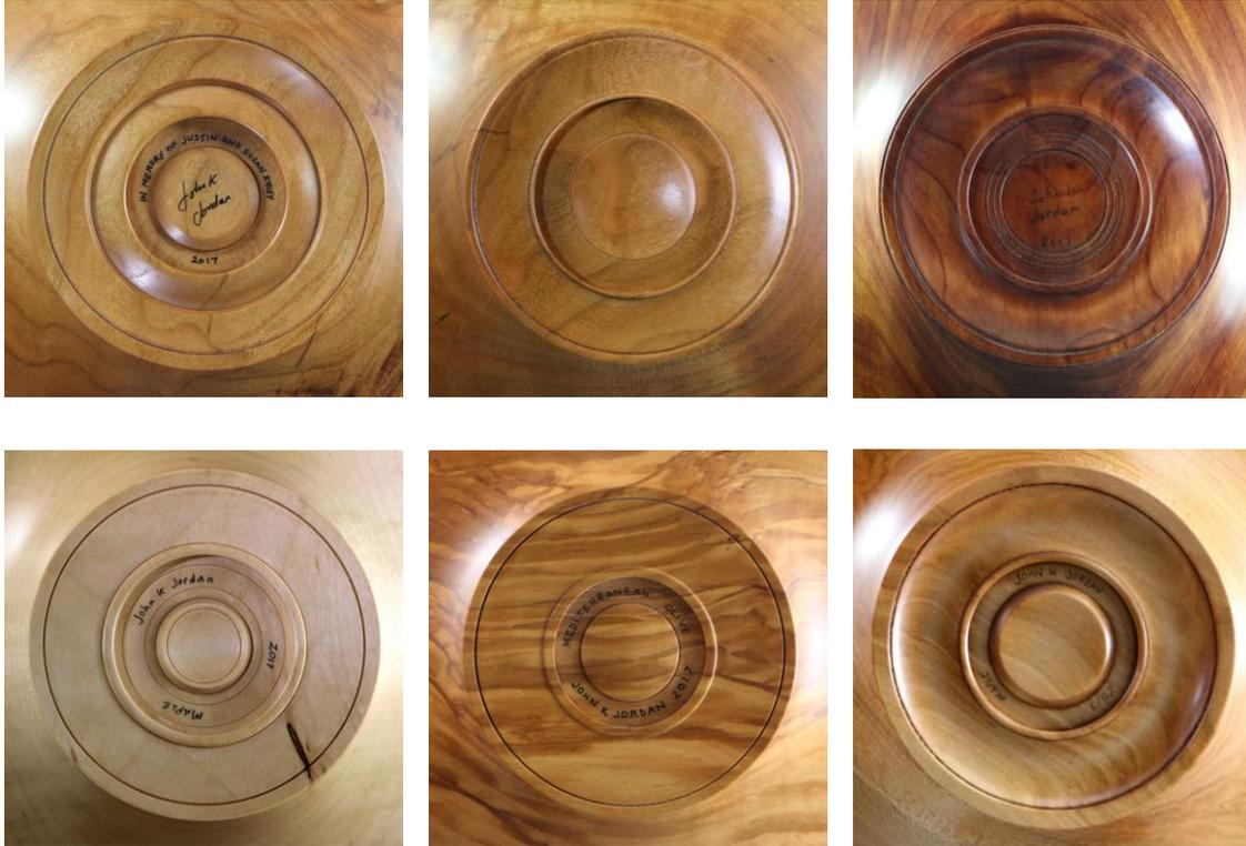
Shape the bottom outside the base ring to create a continuous smooth curve from the base to the rim. A small bowl gouge will work. I've tried various tools and the small Hunter Hercules tool is my favorite.
