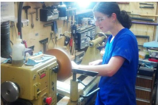
Dish the top in a smooth curve, turning the wings and outer areas parallel to the curve of the bottom. This will make the rim the same thickness all the way across each side. If the dish is too shallow the rim will be thicker in the center.
