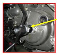
Install the engine turning tool by removing the cover on the left side and inserting the tool, making sure the tangs on the tool engage the indents on the crank shaft. Once the tool is positioned correctly, tighten the retaining bolt snug with a 13 mm wrench.
