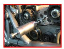
3. Thread the end of the "slap-hammer" into the end of the shaft until finger tight. Slide the weight along the threaded shaft until it hits against the end. Repeat this procedure until the rocker pin moves and the rocker arm has enough clearance to move allowing access to the opening shim.
