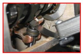
Measurement **A** is recorded in the measurement for the opening shim and the closing shim (for reference).
