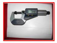
**RECORD** this measurement as **D**, the size of the existing shim.
