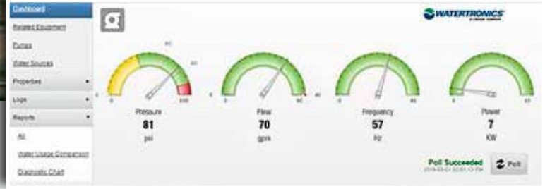
Remote monitoring with AccuDrive delivers real time information by location, including detailed dashboard data and trending charts.
