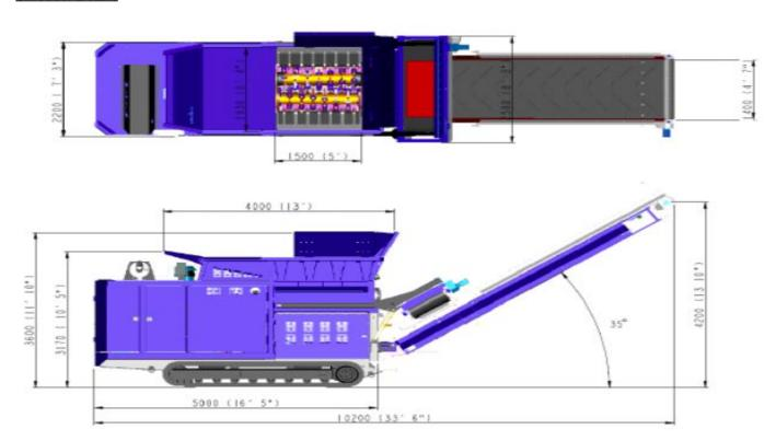
The shredded machinery conveyor feeds the shredded waste directly onto the trommel's in-feed system as part of the next treatment stage.
