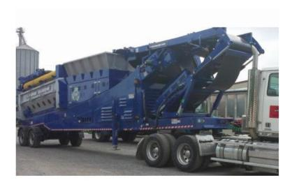
Trommel Machine is also mobile and can easily be transported to different site locations.
