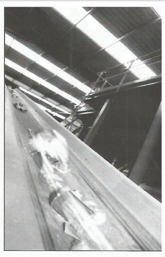
Conveyors start up in cascade sequence with the last conveyor starting first. Conveyors usually run at sequentially increasing speeds to ensure appropriate material levels on all conveyors, thereby facilitating the sorting process whether manual or automatic.
