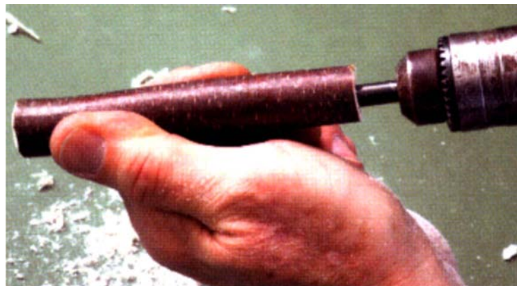
Figure A-2 Drill a Hole
