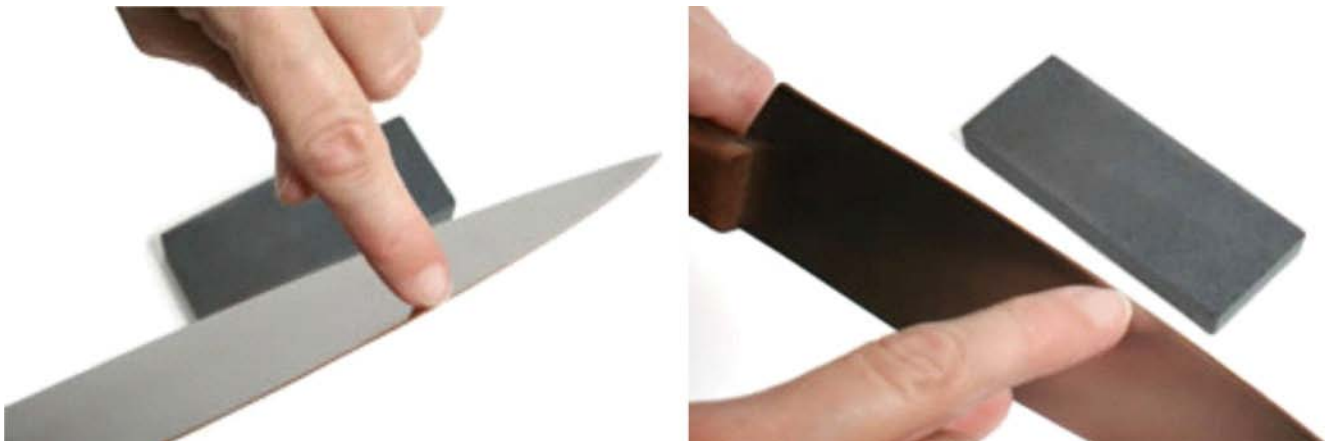
Figure 14 Checking the Bevelled Edge
