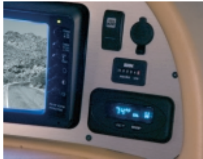
An exterior temperature gauge and compass are now integrated into the dash.
