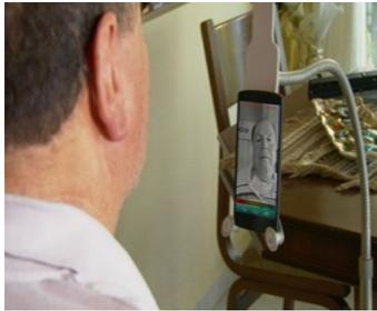
The Sesame Enable Phone is the world's first truly hands-free device that allows users to control a smartphone with head movements.
