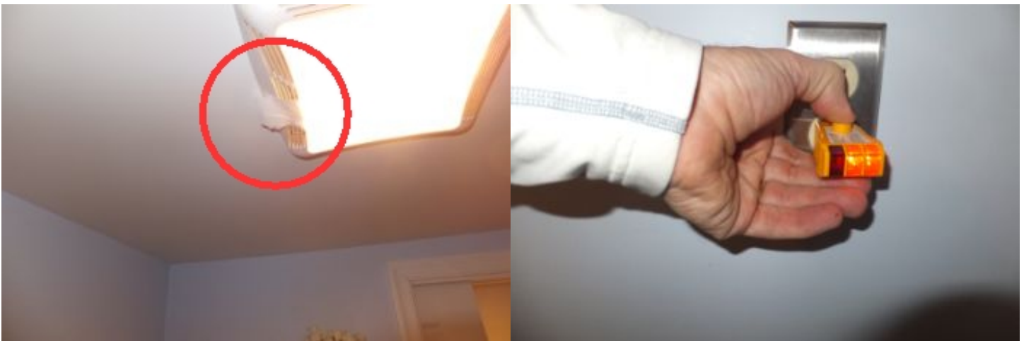
Fan with good ventilation (able to hold a piece of tissue paper)
