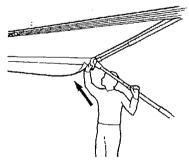
Raise the awning to the desired height by releasing the snap stud on the main arm and pushing up and outward on the roller assembly.
