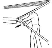
Lock the rafter arm in position by pressing down on the steel main arm bar until the ratchet stud clicks. At this point the fabric will be taut.
