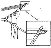
Release the ratchet stud on the rafter arm by pulling outward on the cap. Lift the claw out of the rafter hook. (Pull back, then up)
