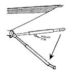
Place the claw casting on the protruding height adjustment stud. To lock the assembly in a travel position, push the other tube downward until the ratchet stud snaps closed.
