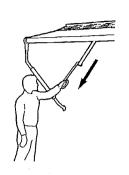
Insert the pull rod into the loop of the center strap and unroll the awning by pulling it toward you. Step under the awning and fold or roll the center strap and tuck into fabric loop. Step 4 RELEASE AND EXTEND RAFTER
