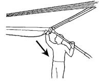
Release the snap stud of the main arm and lower the awning to its lowest position.
