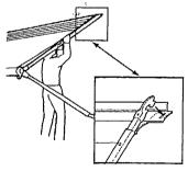
Extend the arm and set the claw shaped end into the slot of the rafter lock.
