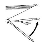
Standing under the awning, release the Rafter arm by pulling outward on the cap of the ratchet stud. Raise the arm upward toward the case.
