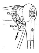
Insert the pull rod into the Z-Lock lever and pull down.
