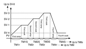
Ramp: the section in which the SV changes toward the target value. Soak: the section in which the SV is the target value, and remains unchanged.
