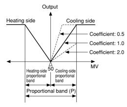
• Before setting the cooling-side proportional band, set the heating-side proportional band to an optimum value. To select the two-position control for the cooling side, set <code>[aal]</code> to 0.0.
