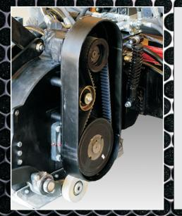
The **TRANSFORMER GRINDER** drum is powered by a hydraulic piston motor connected to the drum by means of a state of the art carbon fiber cog belt. This type of belt is capable of transferring large amounts of power in a very compact size. Carbon fiber belts do not stretch as much as conventional rubber cog belts. That means less maintenance.
