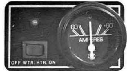
Water heater switch
