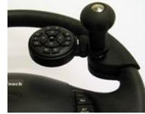
There are also many different types of equipment that can be added to the steering wheel to allow for driving with various types of prosthetic hands or hooks.
