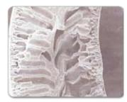
Ultrafiltration (UF) is a technique for separating dissolved solids, suspended solids, bacteria, viruses, endotoxins and other pathogens to produce water with very high purity and low silt density. This hollow-fiber ultra filtration membrane was designed and manufactured to remove suspended particulates, colloidal material, bacteria and high molecular weight material greater than 0.1 micron.
